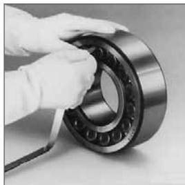
Fig. 1: Checking bearing clearance with bearing on bench.
