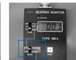
Recording of vibrations caused by a scratch inside a bearing (ENVELOPE)
