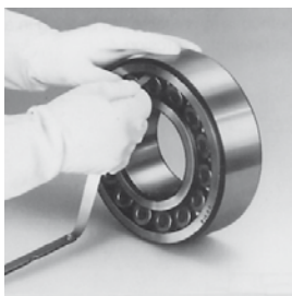
Fig. 1: Checking bearing clearance with bearing on bench.
